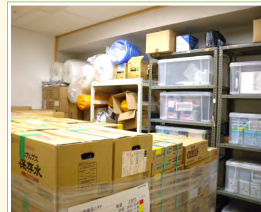
A conference room remodeled into a supply warehouse. The doors were replaced with doors that open out so that the doors would open even if the supplies inside had fallen over.
